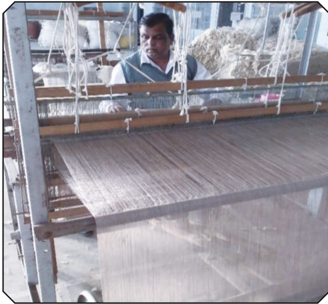
Preparation of lohi from camel calf wool blended fine fiber
